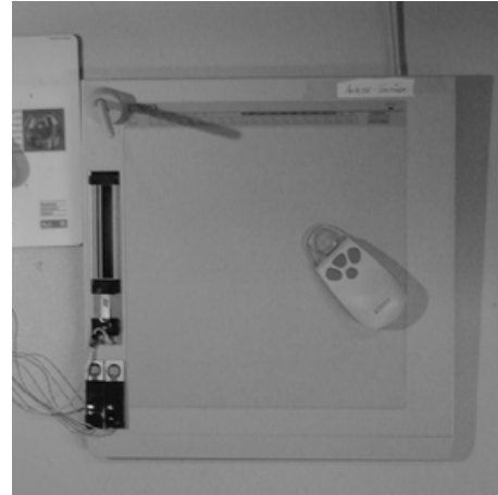
Figure 4: WACOM tablet fitted with additional pressure and position sensors (on the left side of the tablet).
